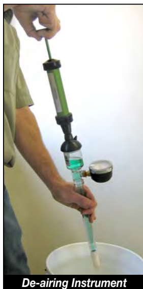
De-airing in the Ground
